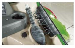
Fendt offers a clever solution for cables that run from the rear of the tractor into the cab. Cables can be guided through the lead-through, no matter what kind of cross section they have. The rear window can be closed, so dust, dirt, water and noise stay outside.
