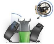
At the headland or during front loading work, you benefit from FendtActive steering\*, reaching a full wheel turn with just one steering wheel rotation. Up to 8 km/h the superimposed steering system is unrestricted, from 8 to 18 km/h the superimposition effect is linear.
