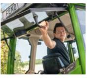
A special feature of the Fendt 200 Vario is the vertical handle on the rear window. which lets you open and close the window from the comfort of your seat.
