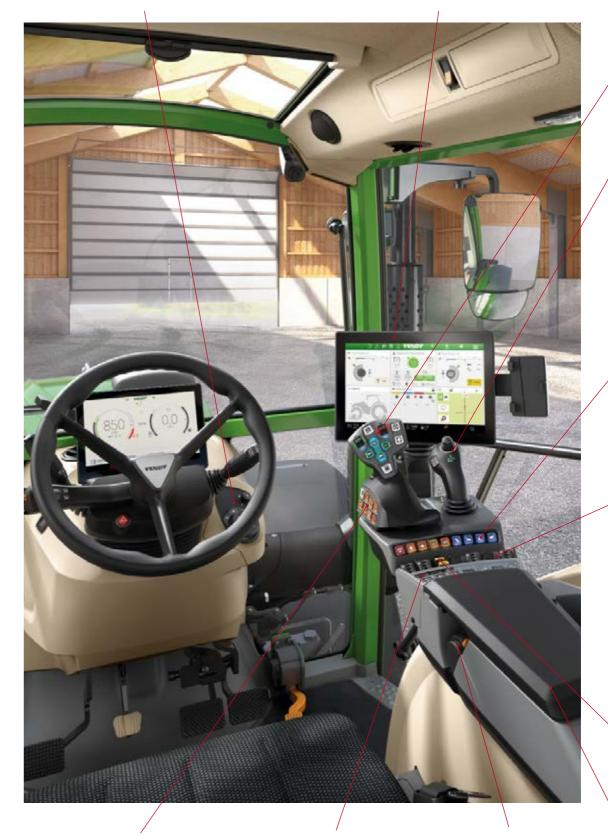
This is where you can easily manage the usual transmission and driving functions with pushbuttons: including two engine speed programs, two cruise control settings and a new dial-controlled active cruise control setting.
