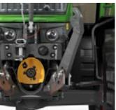
The hydraulic couplings in the rear are neatly aligned and colour-coded. The dust caps close by themselves. For easy coupling, the connections are offset and decoupled under pressure.
