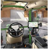
Profi Setting 2 - 3L joystick - 2 linear modules (rocker pair) to control hydraulic valves - 12" terminal
