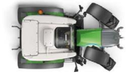
Superbly manoeuvrable due to slender design The wasp-waist design ensures exceptional manoeuvrability and a 52° steering angle (depending on tyres). Its low vehicle weight, starting at 4.1 t, guarantees that soil compaction is minimised during operation.
