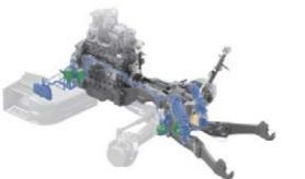
The front power lift is fully integrated and sits tight against the vehicle. This keeps the linked machines highly manoeuvrable. The lower links have a low bottom grip and can be folded for parking. Bellows protect the lifting cylinders against stone impact. The vibration damping fitted as standard prevents bounce and guarantees safe driving and comfort.
