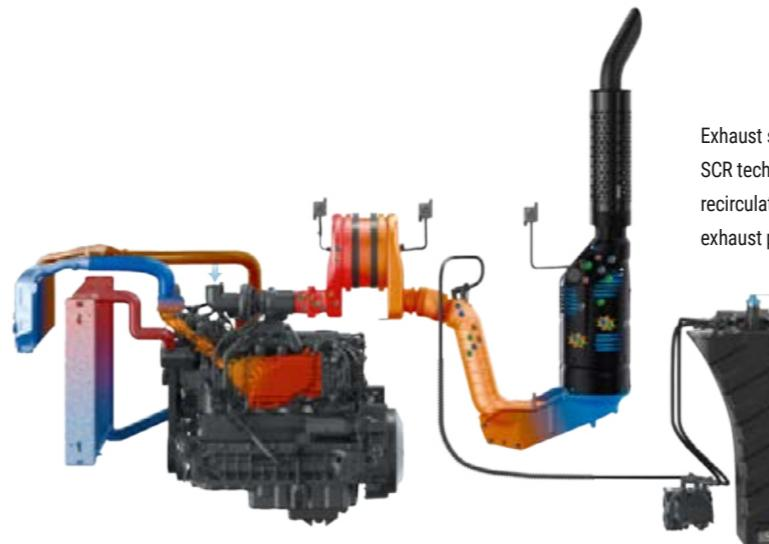
Exhaust stage V is met thanks to the external exhaust gas recirculation, SCR technology and diesel particulate filters. The external exhaust gas recirculation reduces the nitrogen oxides ( $\text{NO}_x$ ) even before reaching the exhaust pipe, so that AdBlue is used particularly sparingly.
