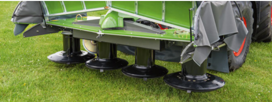
Smooth-running guards which swing upwards make a huge difference to cleaning and maintenance. All Fendt Cutters are very easily accessible.
