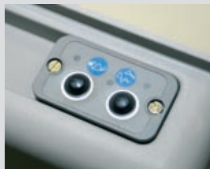
With the Cargo comfort controls, the third control circuit can be switched over to hydraulic attachment lock and the fourth control circuit to the optional damping system.
